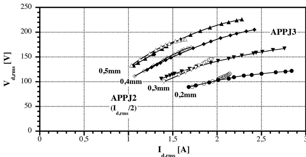
Fig. 2: I-V- characteristics of two APPJs of different discharge area (open symbols APPJ2 72 cm<sup>2</sup>, full symbols APPJ3 36 cm<sup>2</sup>) and gap spacings (0,2 - 05 mm). For better comparison discharge current of APPJ2 is divided by 2.
