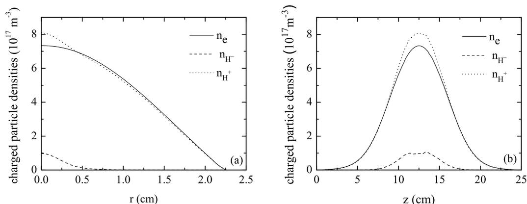
Fig. 2: Radial ( $r$ ) and axial ( $z$ ) variations of  $n_e$ ,  $n_{H^+}$  and  $n_{H^-}$ , the former at  $z = 12.5$  cm and the latter at  $r = 0$ .
