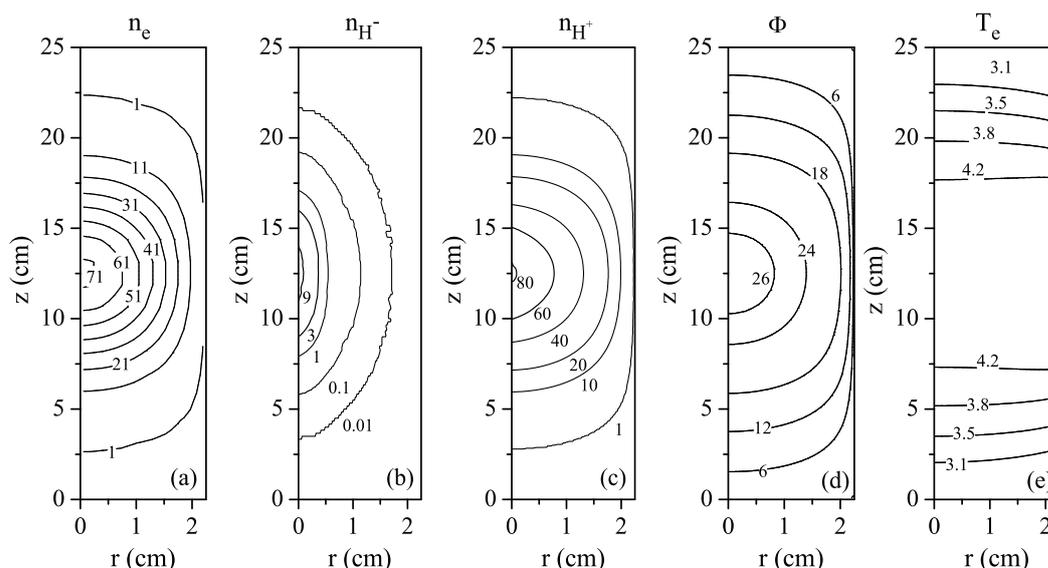
Fig. 1: Contour plots of constant  $n_e$  (a),  $n_{H^-}$  (b) and  $n_{H^+}$  (c) all in [ $10^{16} \text{ m}^{-3}$ ],  $\Phi$  (d) in [V] and  $T_e$  (e) in [eV]. The figures show the modelling domain which is the half of the discharge vessel.
